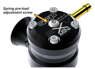
The SXV **DOES NOT** require spring pre-load adjustment to suit specific boost pressures. The pressure-balancing design means that whilst the throttle is open, the pressure on both sides of the piston is equal so it will stay shut under boost REGARDLESS of the spring setting or the boost pressure.
